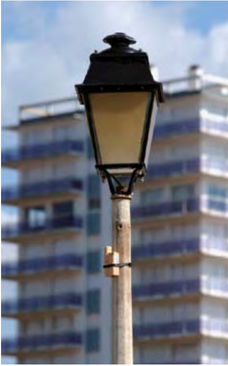
A Yadilys pole-mounted repeater
